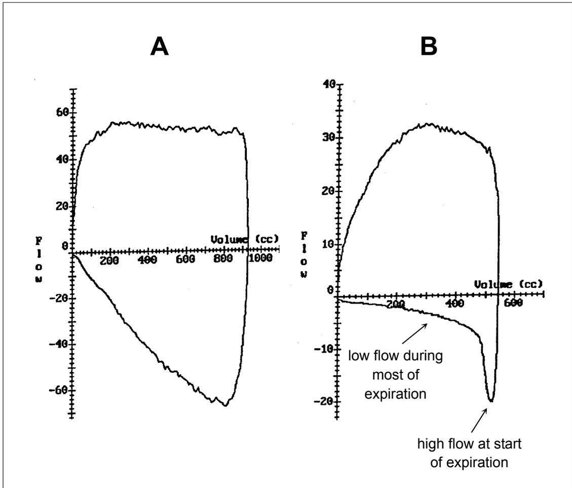
Actual flow-volume loop from a ventilator monitor during volume controlled ventilation of a normal patient (A) and one with chronic obstructive lung disease, COPD (B).
