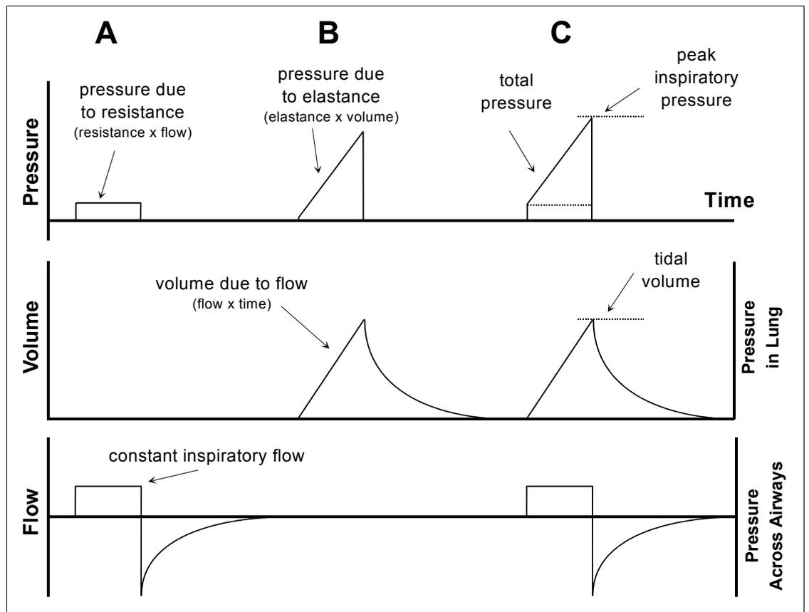
Figure 5-1B shows the results for elastance (the lungs) only. The flow and volume waveforms are of course the same, but the airway pressure waveform is triangular. This is because airway pressure is the product of elastance and volume (a constant and a variable). The result is a graph of a straight line with a slope proportional to the elastance.
